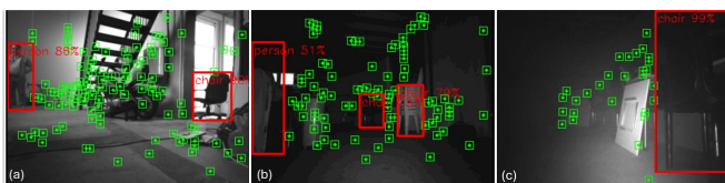
FIGURE 7 Illustration of object detection under different environmental conditions (from left to right): (a) “Light Environment” and (b-c) “Dark Environment” experiments.
